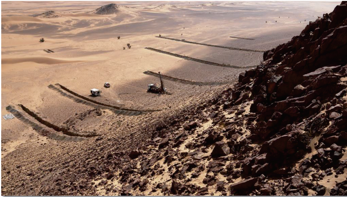
Reverse circulation drilling at Red Hill Prospect, Jibal Qutman.
